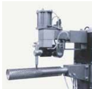
Tube arm For spot welding cylindrical components.
