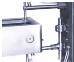
Swivel fitting Welding in hard to reach areas: the electrode holder on the swivel fitting can be adjusted axially; the lower electrode arm adjusted radially and additionally in the height.
