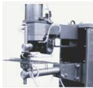
Pendulum and Bar electrode holder Multiple welds in one stroke require (e.g. cross-wires) a pendulum electrode holder above and a beam electrode below.
