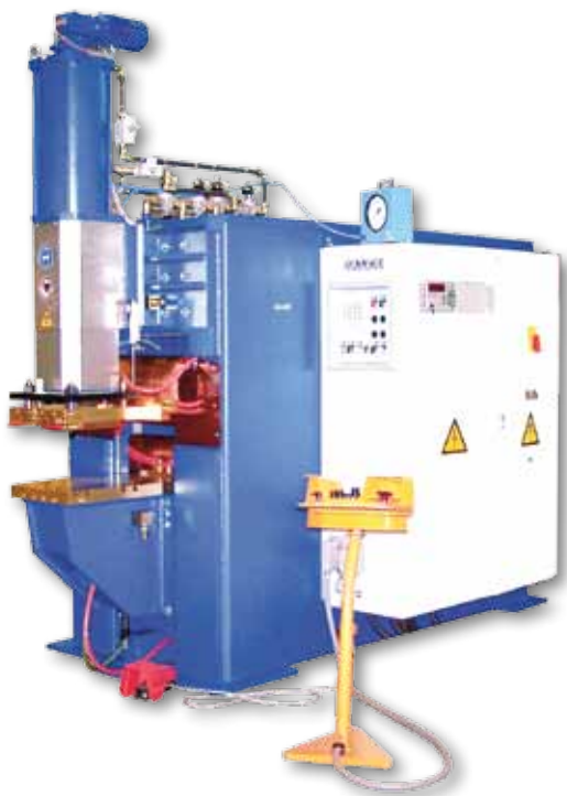
DALEX-3-phase-direct current- projection welding machine type PMS 38-6 G3
