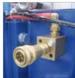
QUICK COUPLING water connection for welding tools
