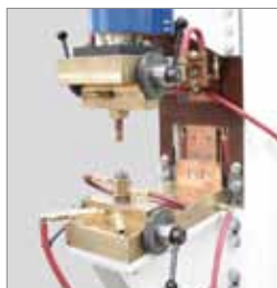
RAPID REETOOLING SYSTEM for quick changing of the welding tools
