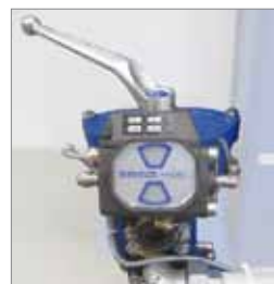
DOUBLE FILTER AND DIFFERENTIAL PRESSURE CONTACT DISPLAY for cooling water
