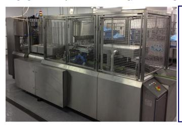
Fully manufactured in stainless steel, Flexi-Pak Inline machines are designed to be very flexible and easy to use. Hygienic designs and open construction also provide easy access. Inline machines are available with continuous motion or index/dwell drives.
