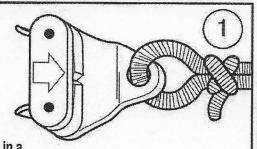
For application in a continuous loop clothesline, put one end of rope through anchor hole and secure with knot. For single line clotheslines and other applications, unit can be anchored with a hook through anchor hole or with screws through holes provided in housing.
