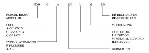
Model **-LM**: Designed for use with grade #2 oil or lighter. No provision for pre-heating oil is incorporated on the burner itself. Standard design includes an oil supply back pressure regulating valve for recirculating oil from the oil inlet on the burner. Pressure atomization is available up to size 300. Air atomization is available for all sizes.
