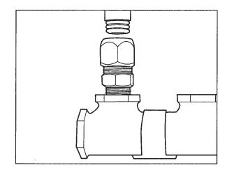
DO NOT USE THREAD SEALANTS WITHIN THE FITTING. USE THREAD SEALANTS ONLY ON THE NPT THREADS.
