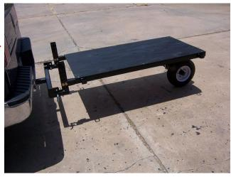
The Hitch Assembly includes two adjustable front mounts. These mounts have a series of adjustment holes. This allows for the leveling of the deck depending on the tow vehicles receiver height. Lowest receiver height is about 10" to the center of the receiver. Once the level position is located, the remaining upright material may be removed if desired.
