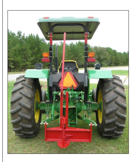
This 3 point lift attachment has a pulling capacity of 10 tons. The handle and hitch are offset for easy visibility from the tractor seat and if you happen to bend a pin, it has been designed for easy replacement. It has been gusseted for strength with a stress proof 3/4" rod and hooks to your tractor with category 2 pins. This is definitely a time and back saver!
