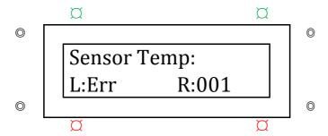
Similarly, when errors occur on roof top or both sensors, the display will indicate as follows:
