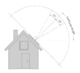
Note: If the above guidelines cannot be achieved, consideration should be given to increasing the solar collection area by adding an extra solar panel, particularly if the direction is further than 45 either side of North. In any case, no direction should be chosen that has any inclination towards South.
