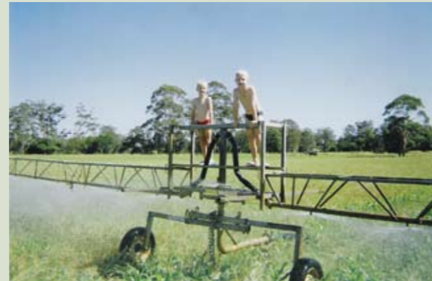
Low pressure boom spray irrigation on summer forage sorghum. Our boys cooling off while checking its operation.
