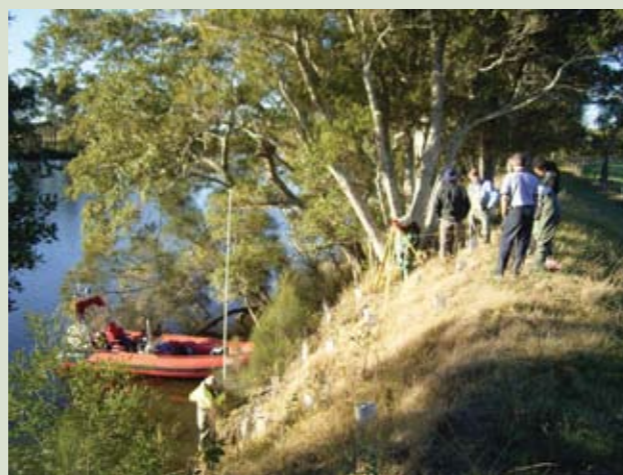
The initial survey of riverbank profiles was conducted with assistance from University of Newcastle and NSW Maritime Authority. Surveying is repeated annually to assess the rate of riverbank erosion.
