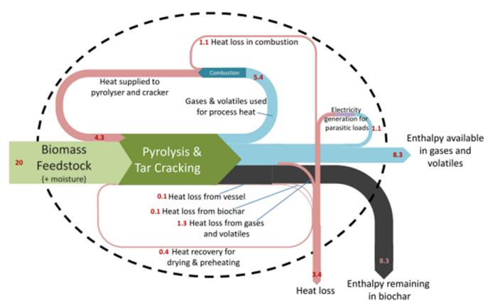
GJ per Mg of dry, ash-free feedstock example system based on slow pyrolysis at 450° C followed by tar-cracking at 800° C
