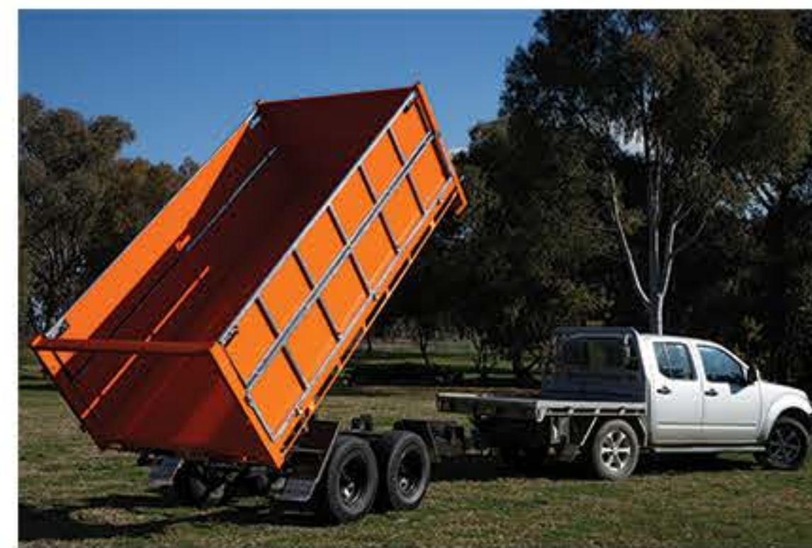
Powder Coat High gloss POWDER COAT finish with Zinc Polymer rust preventative undercoat: High gloss, durable finish
