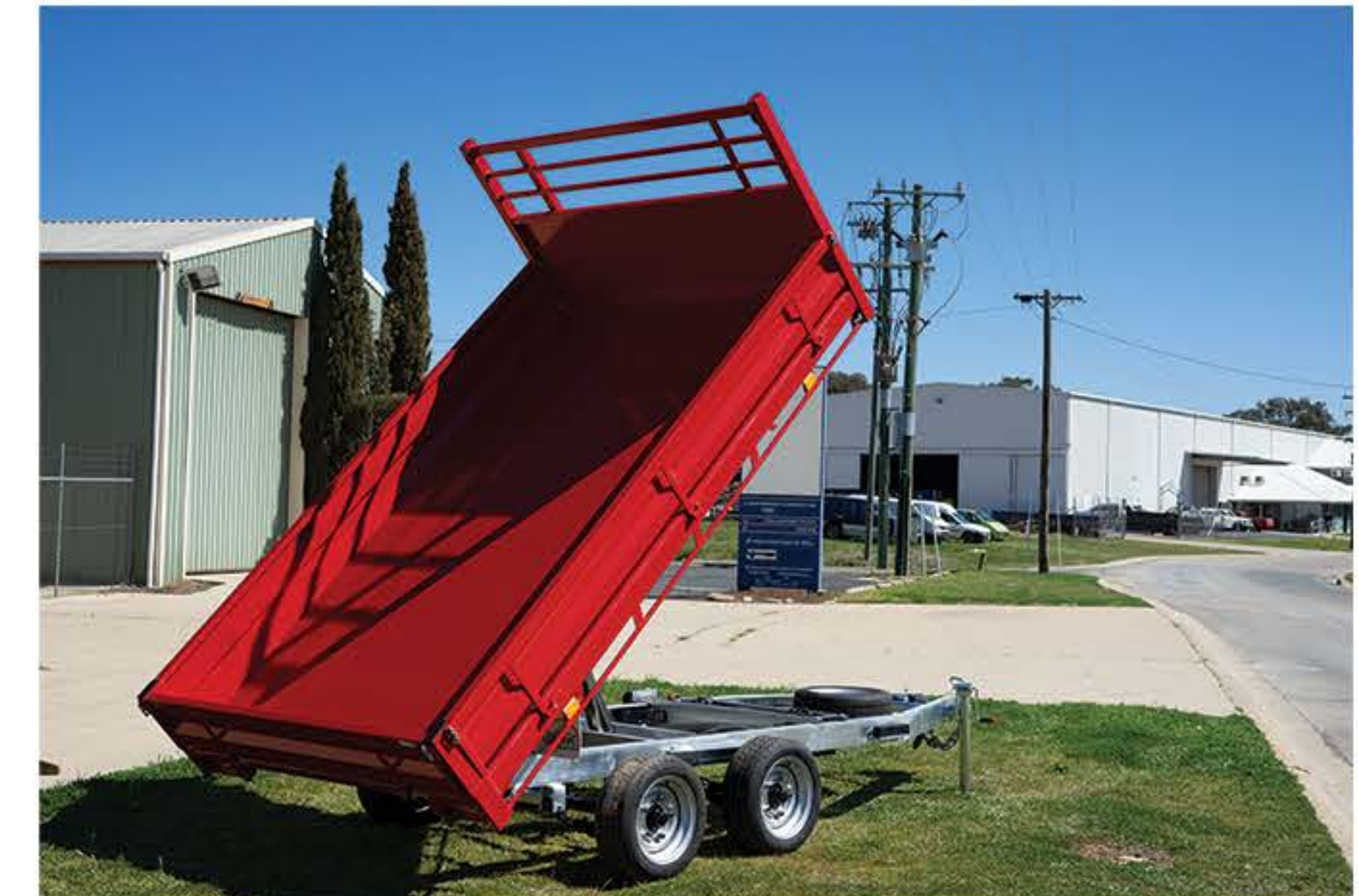
Tray Heights 600T 625mm: 6 Stud Land Rover Wheels & 195/50 R13 Tyres(NEW) 900T 900mm: 6 Stud Land Cruiser wheels & 10R15 tyres: (NEW)
