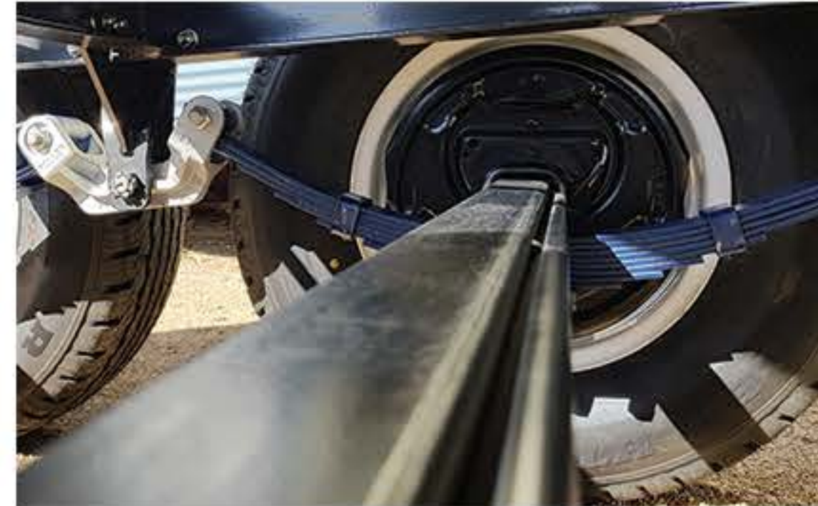
ROCKER ROLLER SUSPENSION (60mm wide, grease able) all Australian made Long life, load sharing suspension With Hardened Pins
