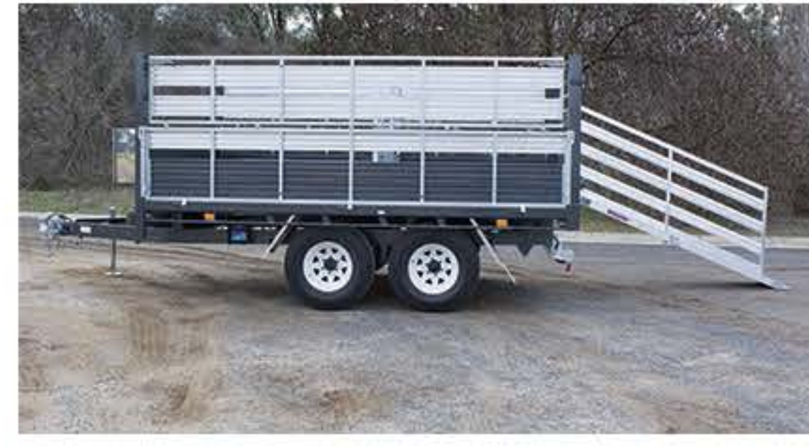
1200mm Livestock Sides Livestock 1.2m double fold side panels with slide & swing rear gate.
