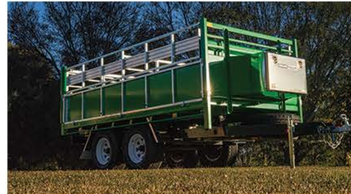
1000mm Livestock Sides Livestock Double fold side stock panels with slide & swing rear gate
