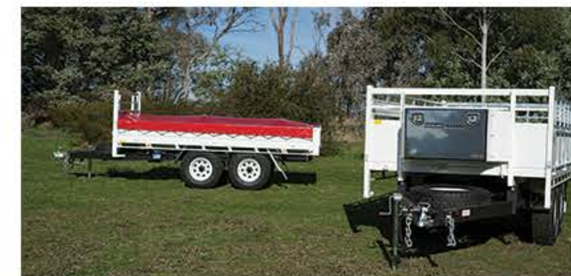
Headboard Mounted Toolbox Stainless Steel Box Mounted to the headboard 800mm x 500mm x 500mm
