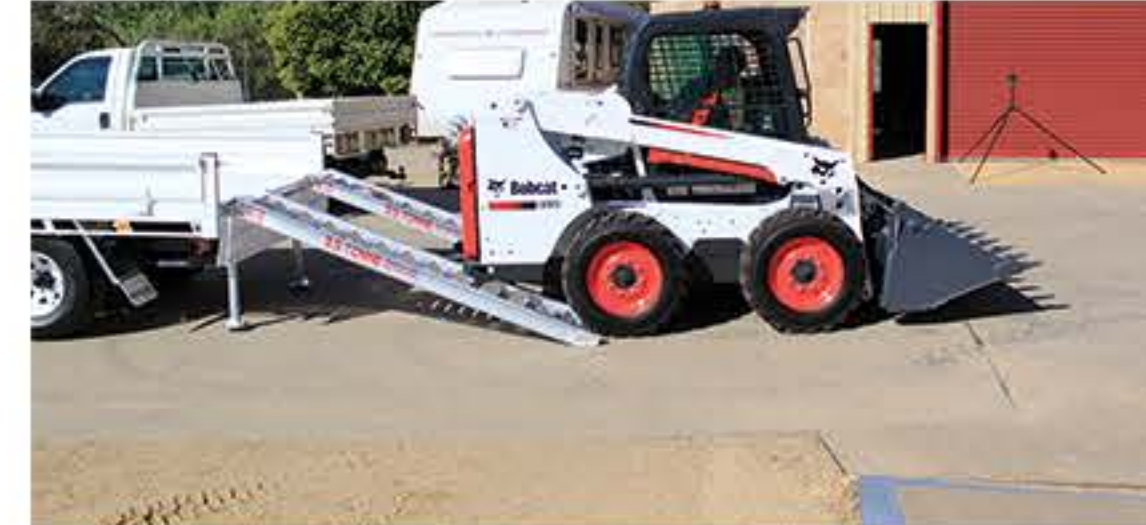
Ramp Options Ride-on mower 2.5 metres 290/340mm 500kg capacity (Folds to 1.4m) ATV 3 metres 340mm 1500kg Livestock Loader 2.5 Metre x 450mm 300kg Machinery 2.5 tonne 3.0 metres 440mm
