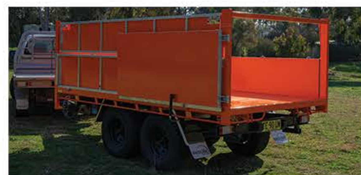
1000mm Builders Sides 1000mm fully enclosed double fold sides with enclosed headboard and swinging rear door
