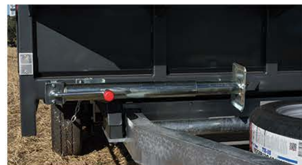
Parking Stand 1200kg parking stand with trans- port mount. A place for everything, no rattle, no lost stands.
