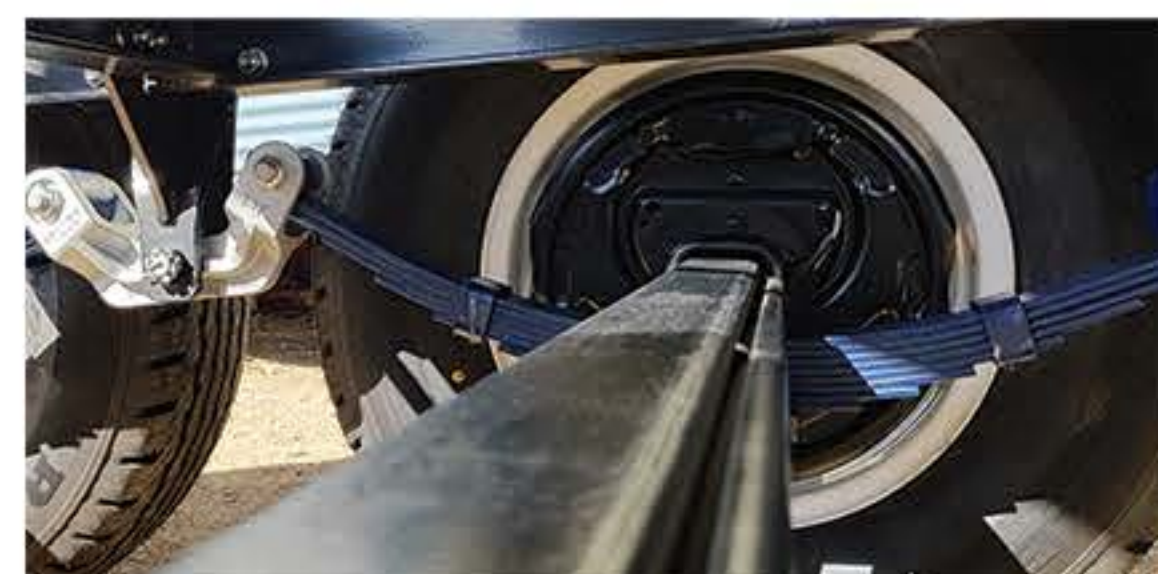
ROCKER ROLLER SUSPENSION (60mm wide, grease able) All Australian Made Long life, load sharing suspension With Hardened Pins
