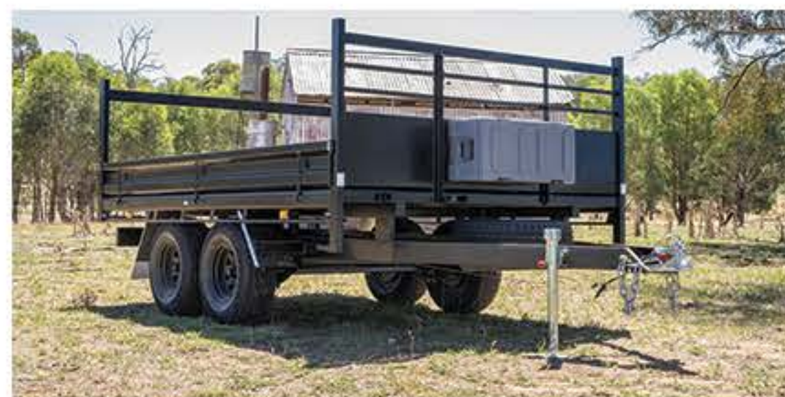
300mm Side Board Set 300mm drop sides with removable rear posts
