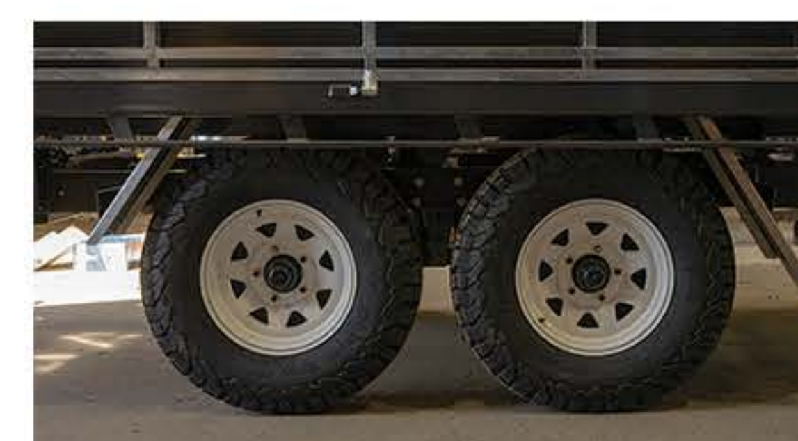
Wheel Upgrade BFG 265/75 R16 Tyres on 5 Stud Landcruiser Rims (set of 5)
