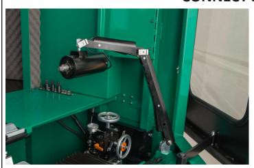
Choose which side of the reel you want to spin from and install the SPIN DRIVE MOTOR with the correct adapter. This will generally be the same drive system component used for backlapping see FIG. 28.
