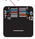
Example: If your reel is a 7" Jacobsen reel you will set the ACCU-REEL POSITIONER as shown above and the relief will be set to the corresponding 12° angle as shown in the picture to the right. If the reel you are grinding does not fit these parameters see Page 38.
