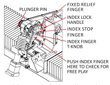
Detail shows Finger and Bed Assembly rotated counterclockwise into relief grinding position (shown without grinding wheel for clarity).
