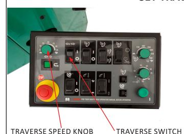
Set the TRAVEL LIMITS of the grinding head by either manually moving the grinding carriage or pressing the TRAVERSE SWITCH to ON and turning up the TRAVERSE SPEED KNOB.
