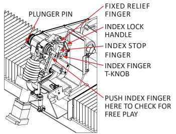
Detail shows FINGER AND BODY ASSEMBLY rotated counterclockwise into relief grinding position (shown without grinding wheel for clarity).
