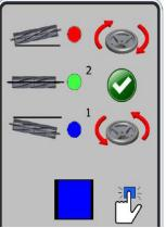
Indicates "Turn the ORANGE HAND-WHEEL clockwise" to move the right side of the GRINDING CARRIAGE towards the operator.
