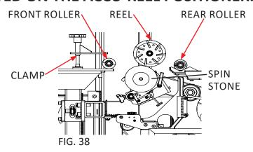
If the cutting unit is not listed on the decal on the left side of the ACCU-REEL POSITIONER you will need to use the POSITION LOCK on the right side of the ACCU-REEL POSITIONER.
