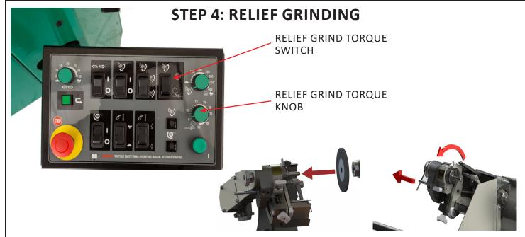
Pull on the left side PLUNGER PIN and ROTATE THE FINGER AND BODY ASSEMBLY up (counter-clockwise, looking from the right side) to the relief position until the left side PLUNGER PIN locks into position. *NOTE:* The PLUNGER PIN must be fully engaged for proper function.
