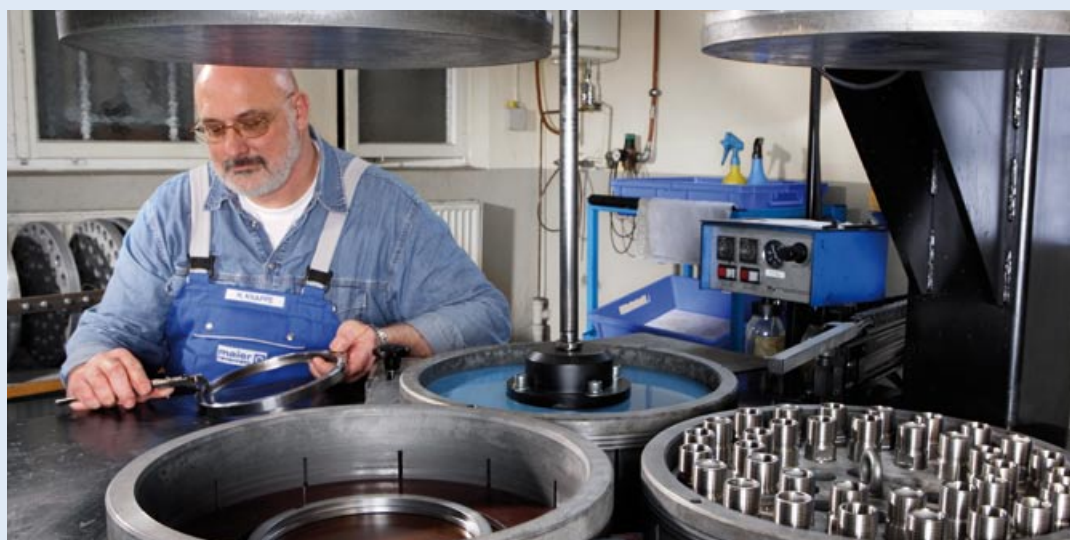
Lapping of sealing surfaces
