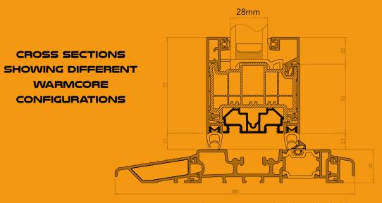
Square sash on Part M compliant low threshold
