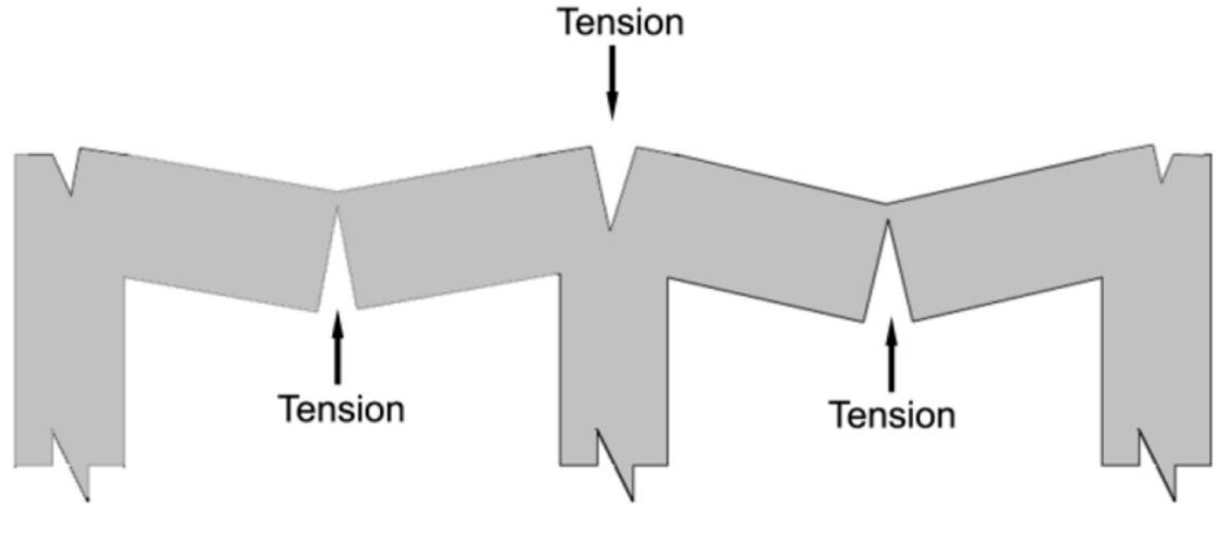
One of the things that happens to a concrete floor, or a masonry wall, is that they are subjected to forces that cause them to flex and bend. Examples
