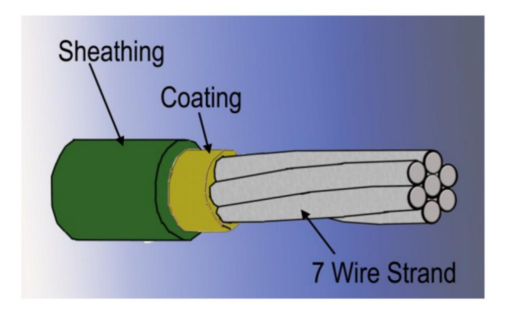
grease is used, the prestressing steel is permanently free to move relative to the sheathing and the tendon is referred to as an *unbonded tendon*. When grout is used, the steel is permanently bonded to the sheathing and is referred to as a *bonded tendon*.
