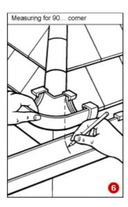
Cut the last length of gutter to the correct size. At the end of the gutter run, fit an external stop end, clipped in place in the same way as outlets, angles and unions. If the new guttering has to join up with an existing gutter, fit the appropriate ogee or half-round adaptor.
