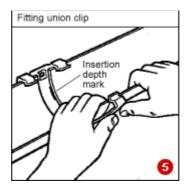
All fittings provide for expansion and contraction of the gutter. When installing the gutter, make sure it does not go past the insertion depth mark in the fitting.
