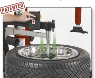
The bead press system speeds and eases clamping, lubricating, demounting and mounting tough wheel and tire combinations.
