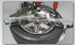
Adding fixed arm allows mounting of the very toughest combinations
