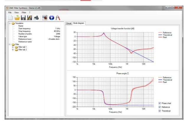
In each diagram two different simulated traces are displayed. The red curve is the simulation based on your library components. The blue curve is based on ideal components. In addition to the attenuation, the phase is displayed in a second diagram.
