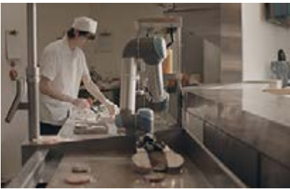
Flippy is a robotic kitchen assistant that uses machine learning and computer vision to cook
