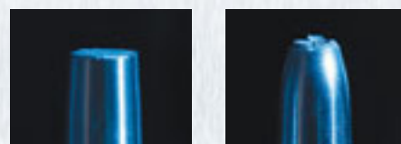
Sprödes Material (Sprödbbruch) / Brittle material (brittle fracture)
