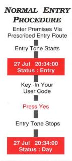
Note 1 PROGRAMMED ABORT Should the user accidentally deviate from the prescribed entry route, the system will automatically change from the 'Entry' mode to the 'Abort' mode if programmed by the installer. The internal sounders will emit a warning tone and the operator has the preset time of 90 seconds to enter a valid access code and return the system to the 'Day' mode.
