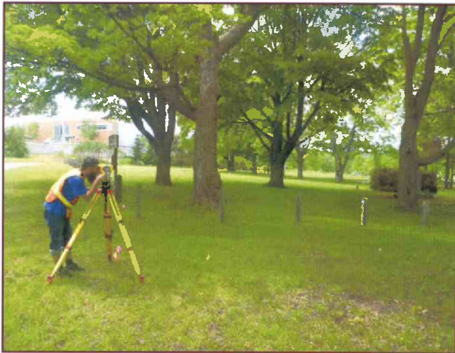
Image 41: Grid Setup Using Trimble Total Station (looking west)
