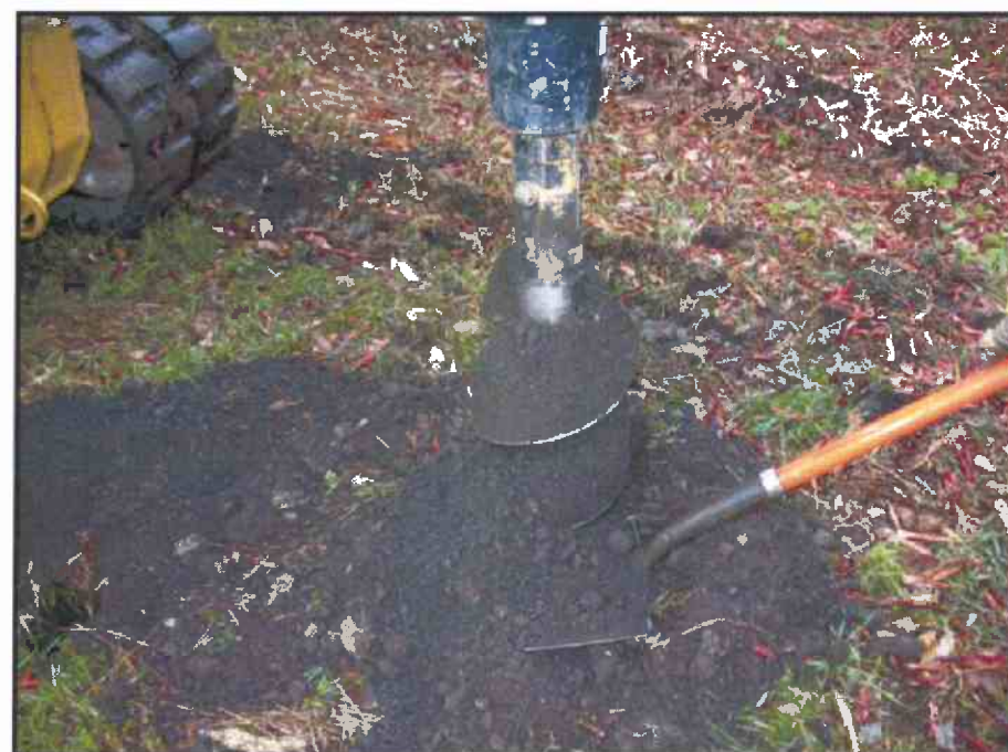
Image 101: Black Cinder-rich Soils Drawn Up by Auger - South Portion of West Boundary
