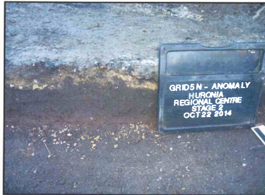
Image 91: Close Up of Asphalt Walkway With Gravel Base and Cinder Beneath - Grid 5 Anomaly Near Datum (looking southwest)
