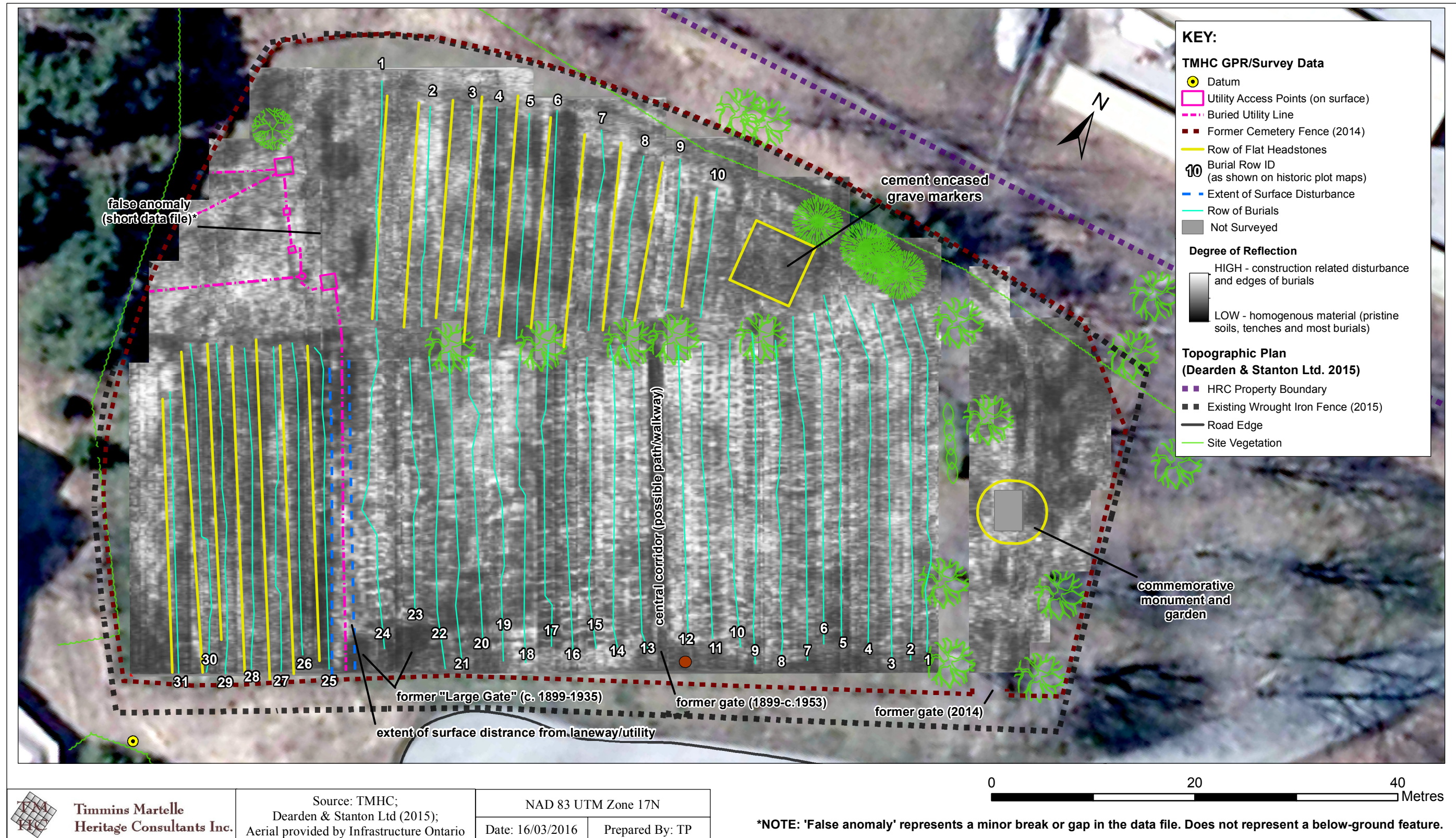
Map 3: Composite GPR Results (Grids 1, 7 and 8; roughly 100, 130, 160 and 180 cm below surface) Shown on Aerial Photography and 2015 Topographic Plan
