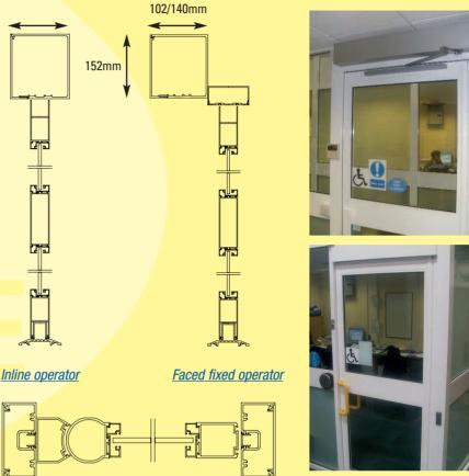
Single swing aluminium door with finger trap protection system
