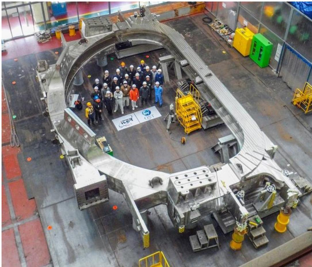
View of a toroidal field (TF) superconducting coil manufactured in Japan. The ITER reactor will contain 18 TF coils, each 17 metres high and weighing 310 tonnes. Half are manufactured in Japan, half in Europe (courtesy of M Claessens).
