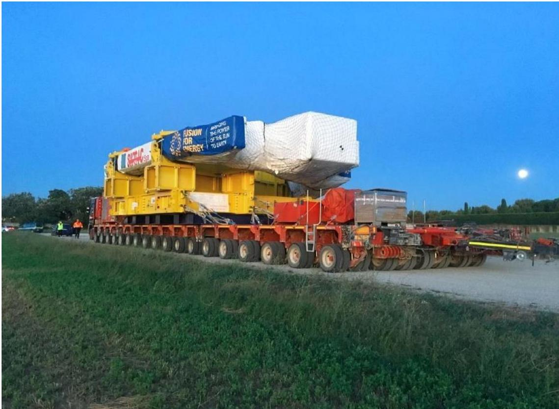
Delivery of one of the large magnets to the ITER site (photo courtesy of M Claessens)
