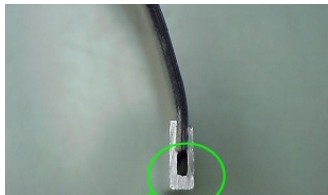
Figure 18: Blanket/Bar not properly installed. Blanket should seat all the way to the back of the bar
