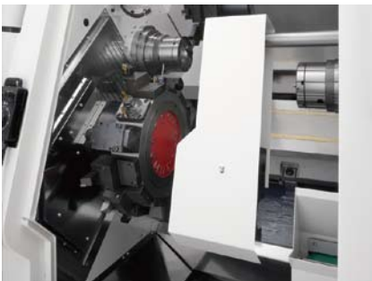
Part catcher Discharges workpiece on to conveyor.
