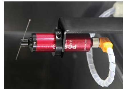
Drill breakage detector Drill breakage is detected by the swing cylinder. The machine stops when breakage is detected.
