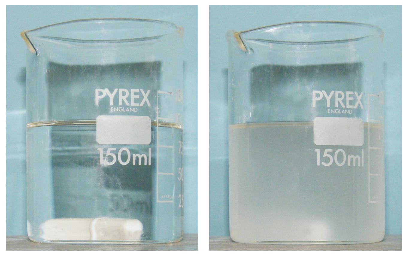
Figure 11.85 g/cm<sup>3</sup> cesium formate with 5% PEG 400 at room temperature (left) and heated to 60°C (right)
