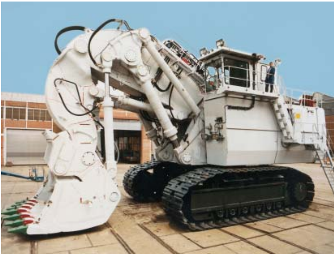
Figure 4: O&K hydraulic excavator RH 400: Load bearing structural components made of DILLIMAX 690 T (Illustration with the kind permission of the Orenstein & Koppel AG, Dortmund, Germany)
