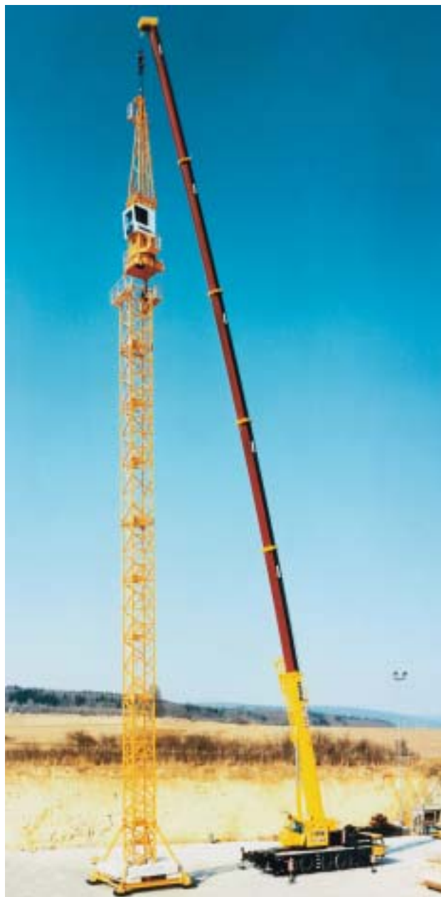
Figure 20: Mobile crane assembling a tower crane (Illustration used with the kind permission of Liebherr-Werk Ehingen GmbH, Ehingen, Germany)
