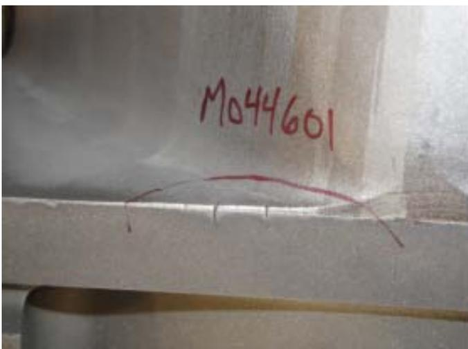
After sectioning the buckets the internal and external coating and surface condition was metallurgically evaluated at 2 airfoil cross sections 1½” from the tip and 1” above the
