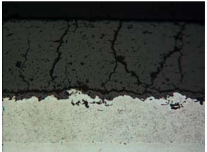
Figure 8, Repaired bucket with non DVC TBC coating
