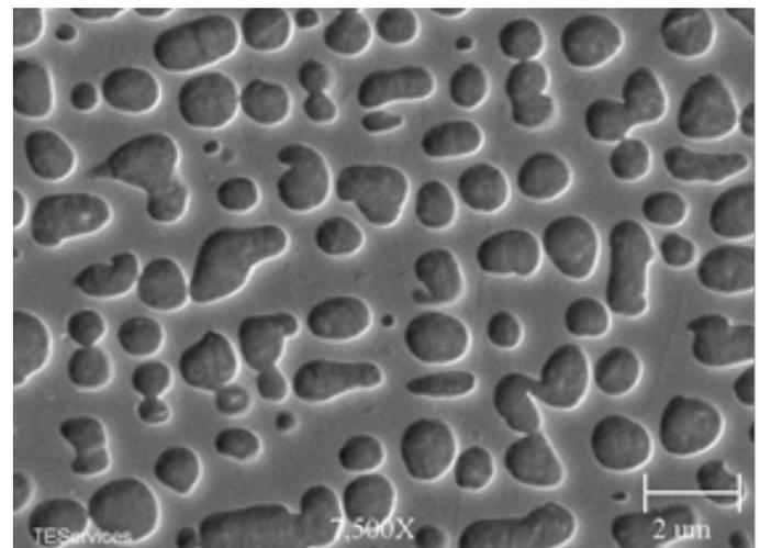
Figure 11, SEM 7500X 2<sup>nd</sup> cycle bucket at TE tip
