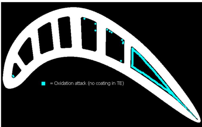
The condition of the buckets was further investigated using visual and Scanning Electron Microscopy (SEM) at 5 locations: TE tip, LE 1/3 from tip, cross and longitudinal mid sections 2/3 from tip, and root, figure 6. Some large secondary metallic phases were observed at all buckets and at all locations and these were titanium and tantalum carbides that were formed during the original casting manufacture- see figure 10.
