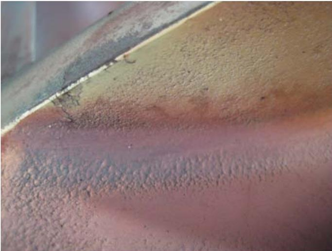
The bucket that completed 1st cycle and 2nd cycle were also Non Destructive Tested (NDT) including Penetrant Testing (PT) and visual after stripping of the coating – see figures 4 and 5. The results were compared to the simulations and confirmed the earlier results in most cases, the simulation was further defined in other cases as shown in figure 3.
