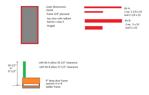
Featuring R-16 Insulation, solid 3/4" wood construction, hinged for convenience, weather stripped, ready to install. Frame dimensions: 11" tall X 25" wide X 53 3/4" long, matching exactly the standard 24X54 attic frame. Includes spacer kit, discard if not needed.
