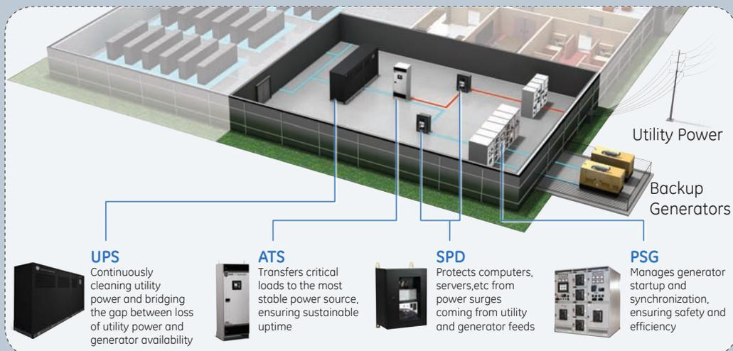
For mission critical processes, customers rely on our Digital Energy's industry-leading power quality solutions to increase critical system reliability. Power Quality has technology that delivers superior performance and industry-leading energy efficiency for facility backup power management. In addition to our UPS Solutions, we provide the Standby Generator Paralleling Switchgear, Automatic Transfer Switches and Surge Suppression Devices that deliver power efficiently and reliably.
