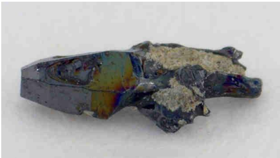
Figure 1. The largest known natural moissanite crystal, found along the Kishon River in north-eastern Israel, measures 4.1 mm in its longest dimension. Photo by Vered Toledo.
