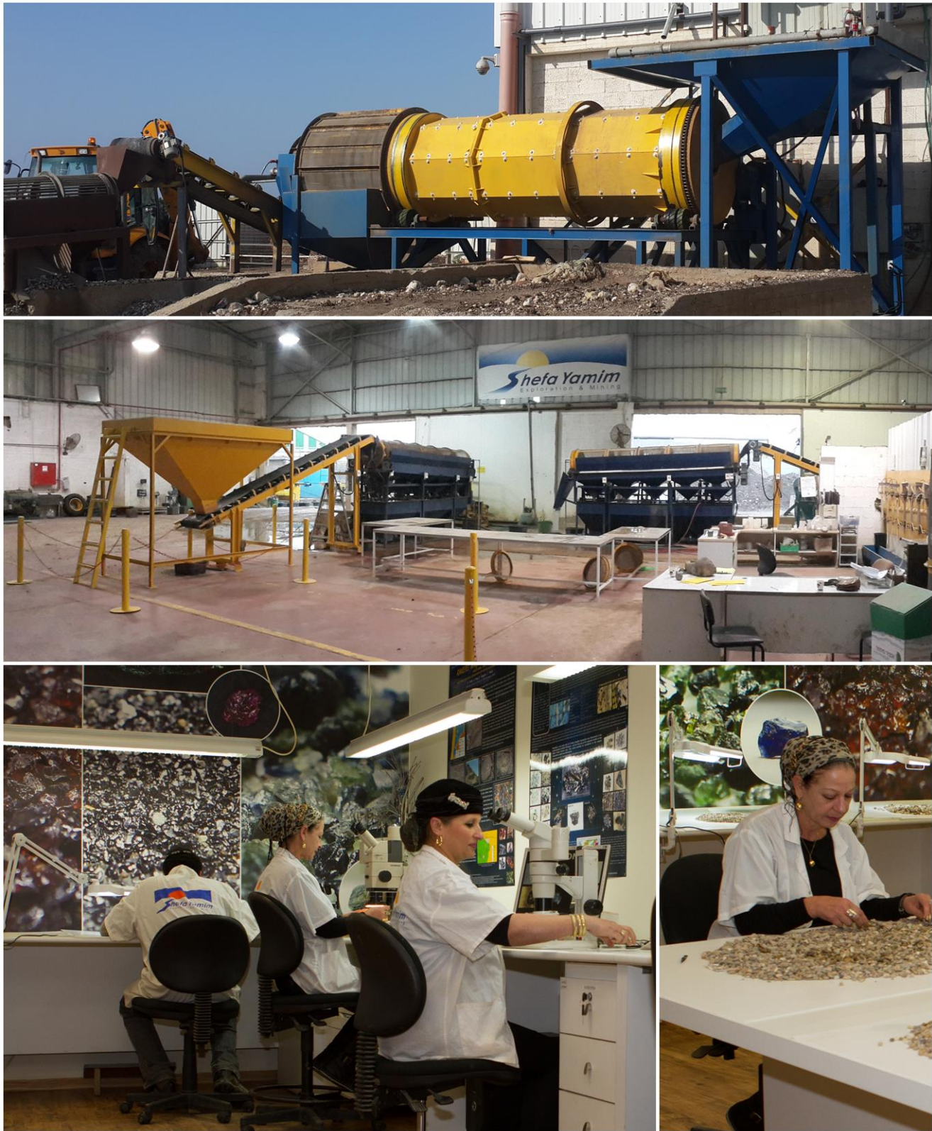
Figure 49: Processing facility and laboratories at Akko. Top: Scrubber plant for the washing and liberation of sand-size sediment from clay aggregates. Middle: Two classification and jig plants. Bottom: Mineral final recovery laboratory where the sorting of minerals is done manually.
