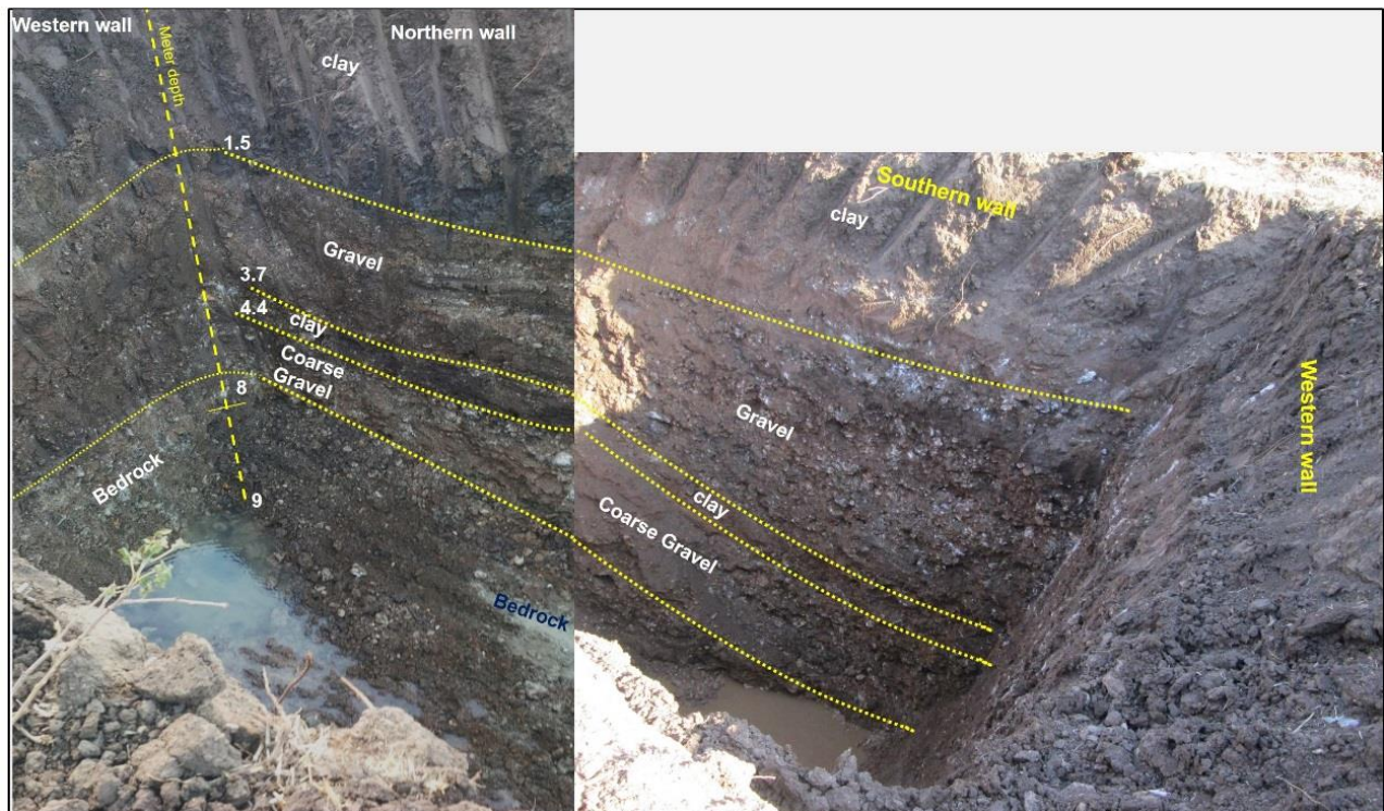
Figure 31: Bulk sample SY-1125 excavated down to bedrock some 8m below surface.
