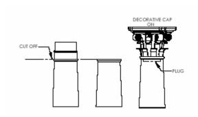
The decorative capitals are load bearing. The total height listed in the brochure should be added to the shaft less the cut off in order to determine the maximum possible length for each column/capital combination.
