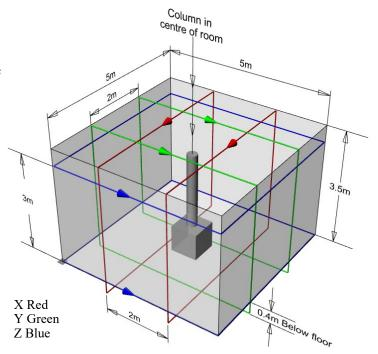
practical for new-build labs. Parts of the bottom Z cable also need to be buried at door openings.
