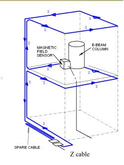
from Spicer Consulting. The joints are insulated to ensure that there are no shorted loops in parallel with the cables. Similar precautions must be taken if the frame is obtained locally, otherwise the cancelling performance will be compromised.
