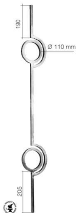
Art. 1091/2 \varnothing 12 mm L 135 mm H 1000 mm
