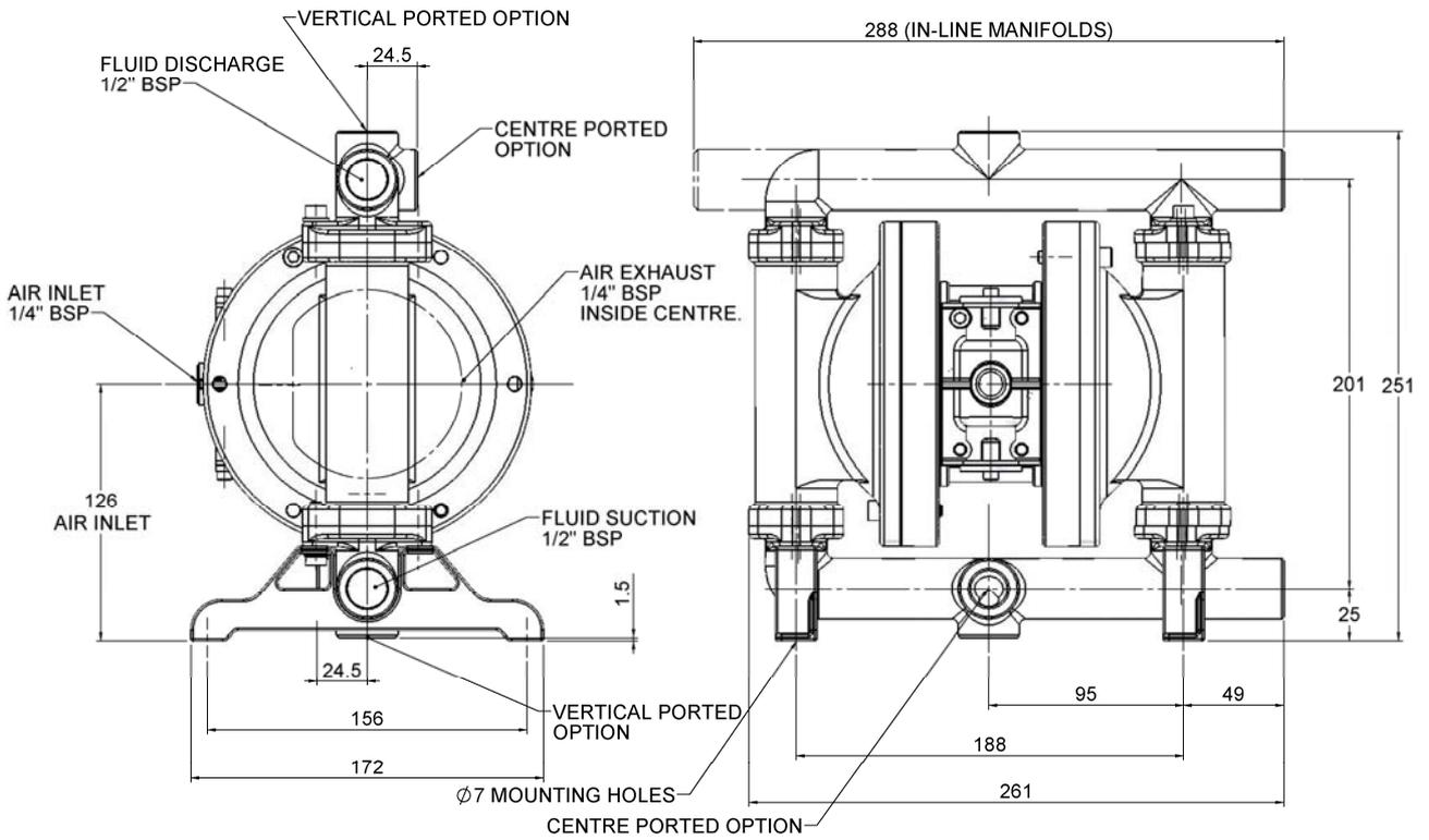
General Assembly :- B15 Stainless Steel / Aluminium pump, all dimensions +/- 2mm
