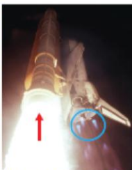
Hydrocarbon flames (left, red arrow) vs. hydrogen flames (right, blue circle)
