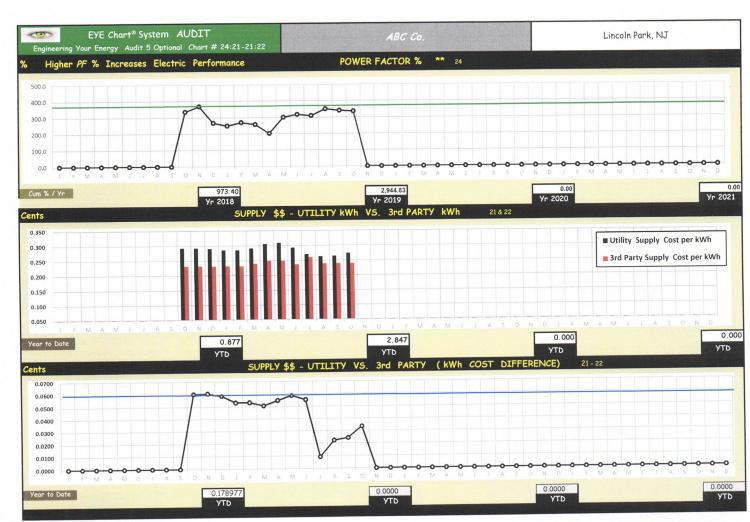
\*\* Power Factor (pf) High pf % increases efficiency of electric power to do more useful work. PF is the ratio of real power and apparent power in a circuit. A lower pf indicates an inefficient product as it draws more current into the electric circuit than is utilized by the electric load. The more current in the transmission lines lead to more power lose in the form of heat.
