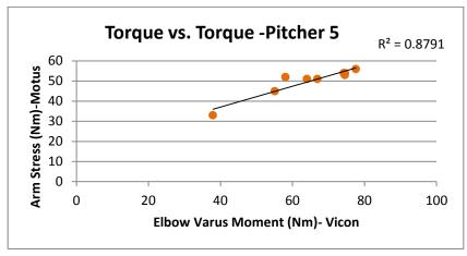
Figure 5: Pitcher 5 results of the Vicon measured elbow varus moment (x-axis) to the Motus Sleeve Arm stress measure (y-axis).
