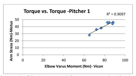
Figure 1: Pitcher 1 results of the Vicon measured elbow varus moment (x-axis) to the Motus Sleeve Arm stress measure (y-axis).
