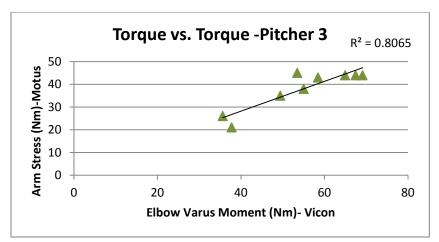
Figure 3: Pitcher 3 results of the Vicon measured elbow varus moment (x-axis) to the Motus Sleeve Arm stress measure (y-axis).
