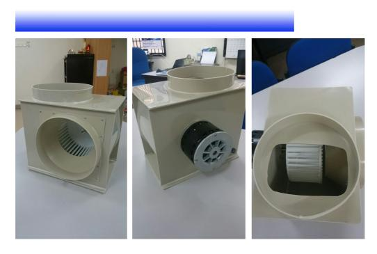
Our PP centrifugation fan is made of PP material, it's suitable for poisonous or corrosive gas with temperature within -8 degree to +80 degree. It's for interior room use only. The fan is driven by motor directly. We use many measures to prevent corrosion for transmission shaft or motor. It's a single phase motor with 3 different rpm to adjust the wind volume.
