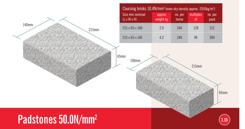
We produce a useful range of padstones. Manufactured to a 50 N/mm<sup>2</sup> compressive strength, they are suitable for the majority of applications where a high-strength bearing pad is required – such as under steel joists. The padstones are produced in a range of sizes designed to fit most block and pier dimensions.
