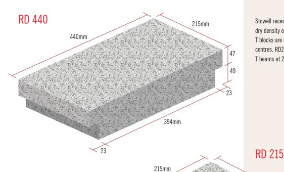
Stowell recessed T blocks have a nominal ovendry density of 2000kg/m<sup>3</sup>. RD440 recessed T blocks are used with T beams at 514mm centres. RD215 recessed T blocks are used with T beams at 289mm centres.
