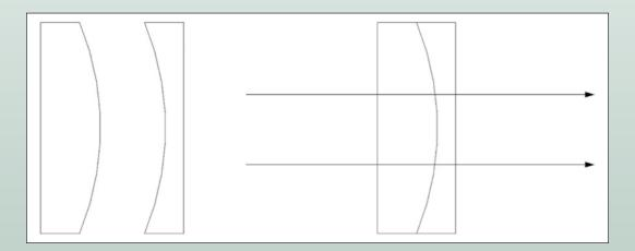
This configuration creates a Gaussian Compensator or Apodizer – a filter that changes the Gaussian distributed intensity profile to a flat top distribution.
