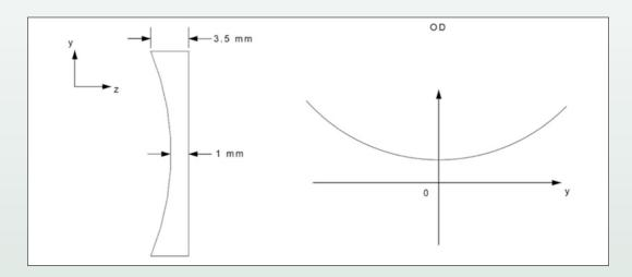
The plano-convex filter glass introduces optical power into a traversing beam of light and can have a dual function as a lens and filter combination. If this is undesirable, optical power can be eliminated by using a clear glass lens of equal but opposite power adhered to the filter glass lens with optical cement as shown in the figure below.
