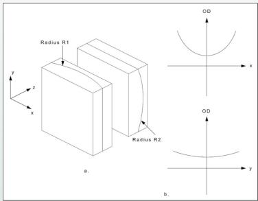
In preliminary work for a military application we were given a very specific optical density profile. We designed (but never built) a filter that matched the OD profile using a section of a sphere, the fabrication process shown devised in the figure to the right.
