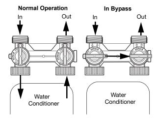
Figure 6 Typical Globe Valve Bypass System
