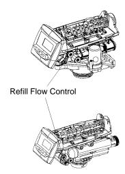
If the brine tank is not refilling correctly (too much or too little water) the refill flow control should be cleaned and inspected.
