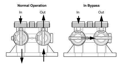
Figure 5 Autotrol Series 1265 bypass for use with Performa and 1100 valve bodies
