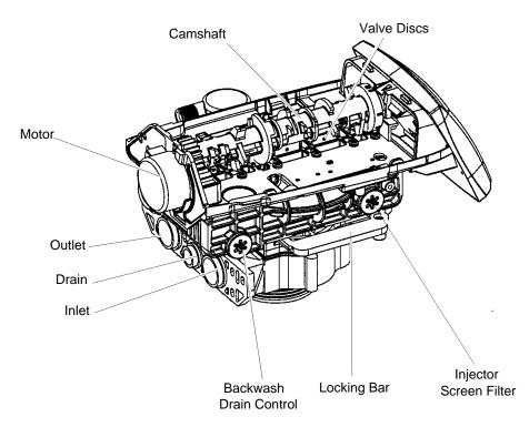
Figure 2 Performa Valve Identification
