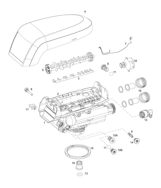
Warning: Do not use the flow control ball with #10A.
