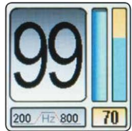
The number recorded is the lowest noise level taken (on a scale of 0 to 99) during this period that is relevant for leak detection. This information is also shown in bar form to the immediate right of the number.
