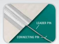
Connecting pin installation can be difficult, given both the small diameter of the pin and the flexibility of the material. Io ease and speed this process we offer Leader Pins, which attach a smaller diameter, rigid lead pin to the larger diameter, flexible connecting pin. The lead pin is easily fed through the splice, allowing the actual connecting pin to be pulled through. The use of Leader Pins often reduces pin insertion time by more than 75%.
